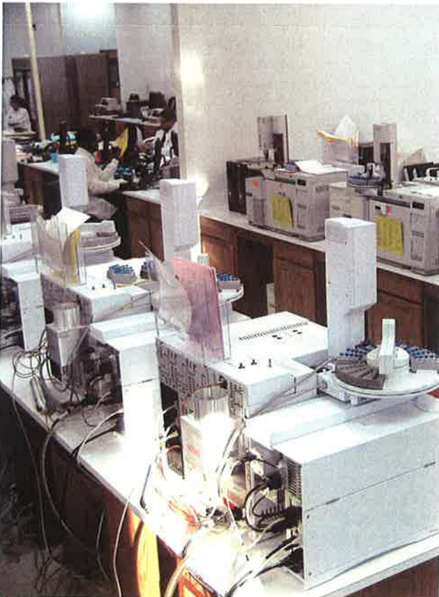
Above, Clinical Reference Laboratory, Inc. (CRL) processes urine samples for analysis using Gas Chromatography Mass Spectrometry (GC/MS) instruments. There are 27 GC/MS instruments in the toxicology laboratory at CRL.
